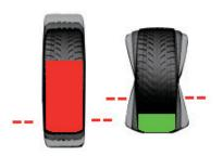
SmartWeight® panel displays wheel balance condition
