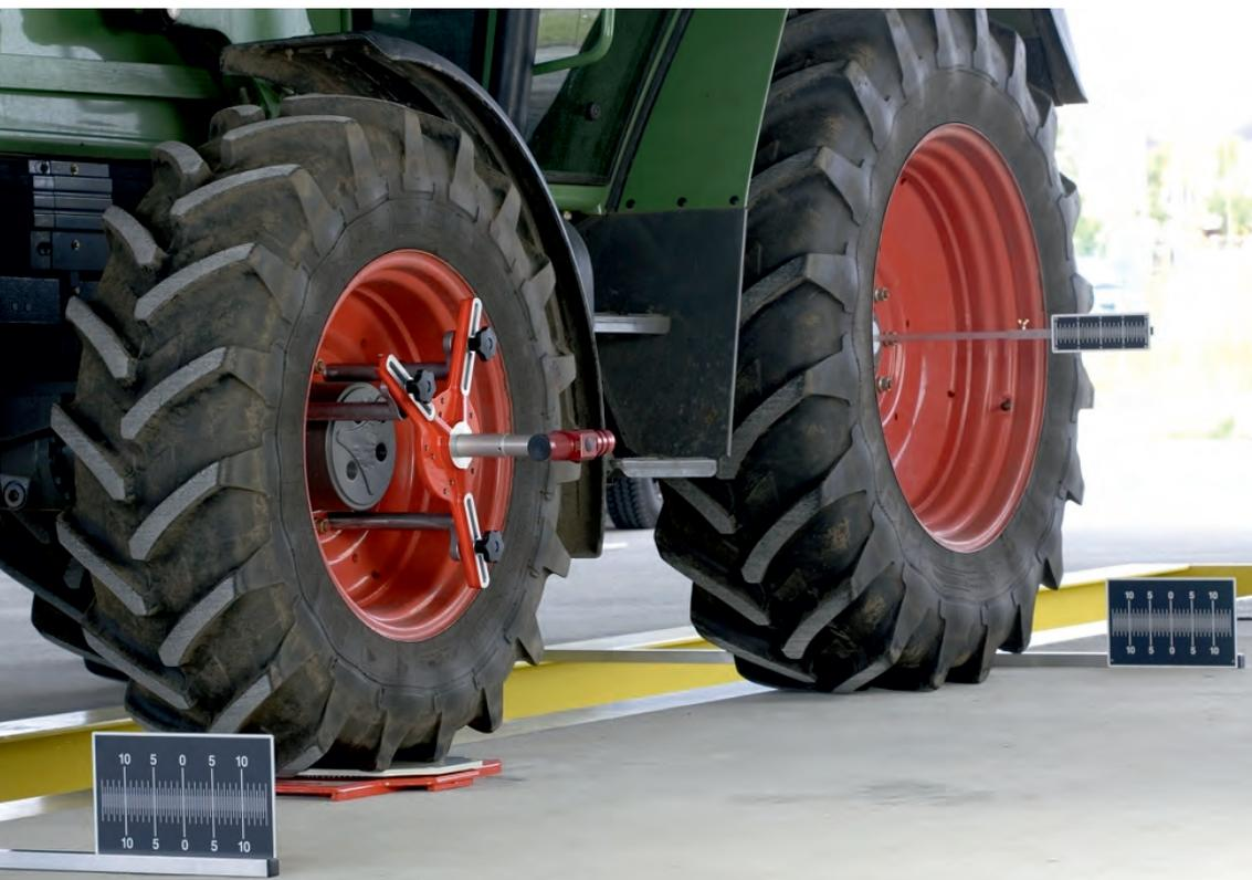
Toe alignment in modern tractors and agricultural machinery is as important as in cars and utility vehicles.
