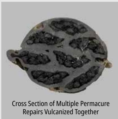
Cross Section of Multiple Permacure Repairs Vulcanized Together
